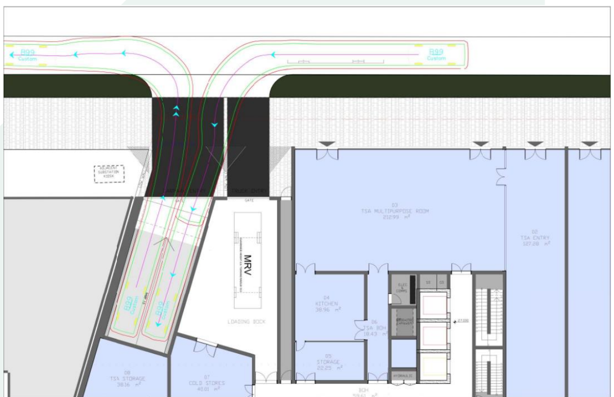
Figure 2: Loading Dock Area. Direct Access Via Willock Ave
