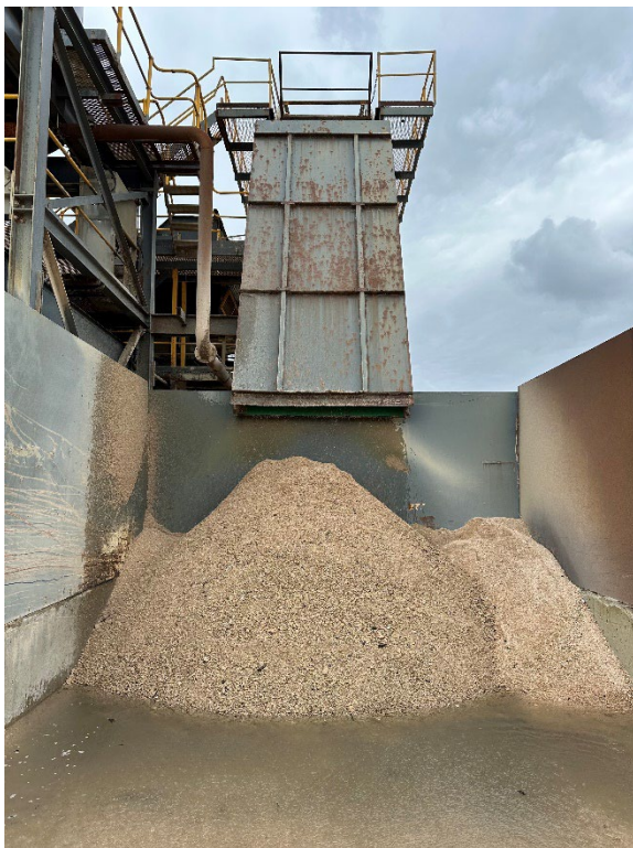
Photograph 1 Accumulation of overs at the sand washplant on Lot 2 South
