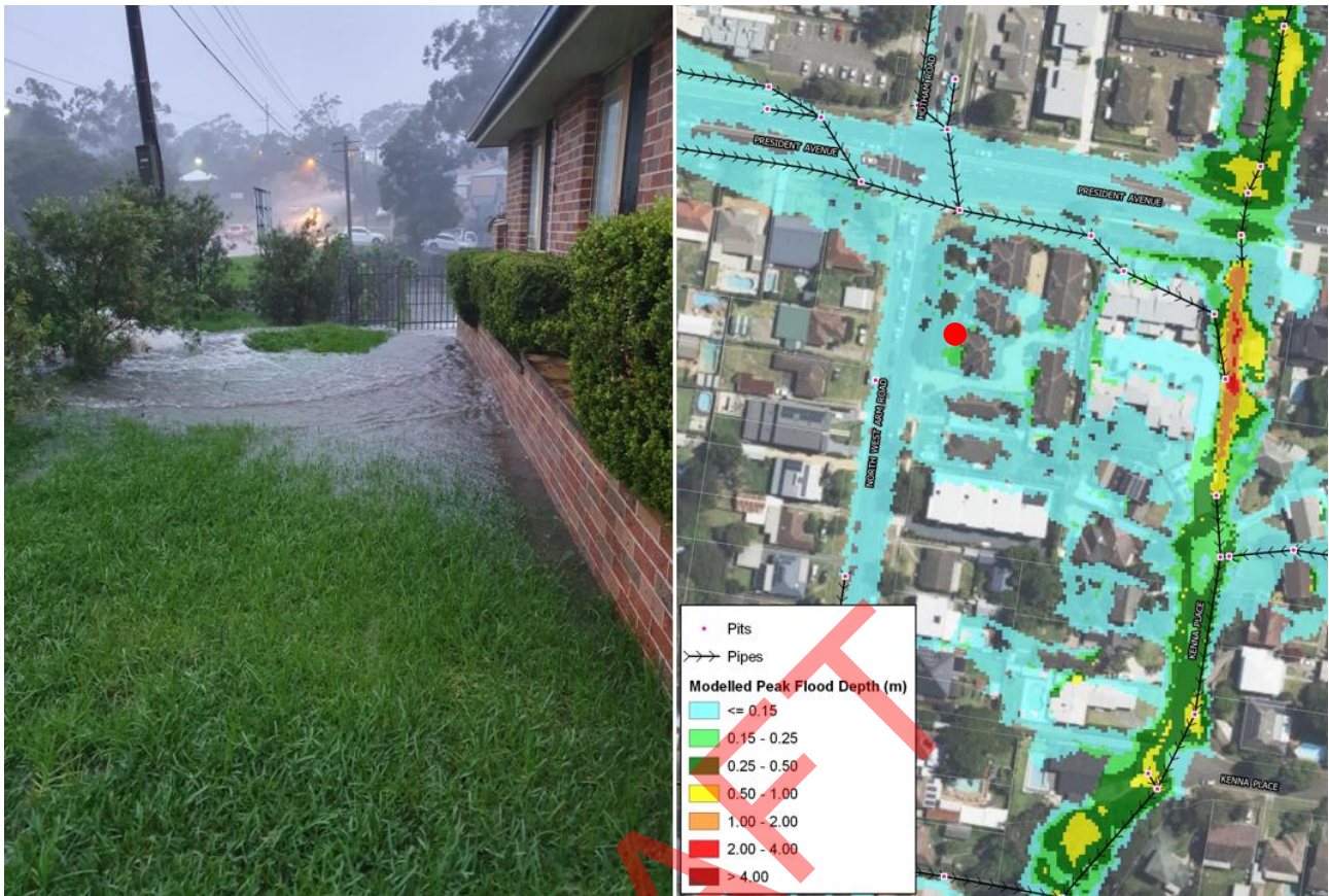
Figure 5.5 Photograph and Predicted Flood Depths for February 2020 Event – Corner President Avenue and North West Arm Road (GyMEA)
