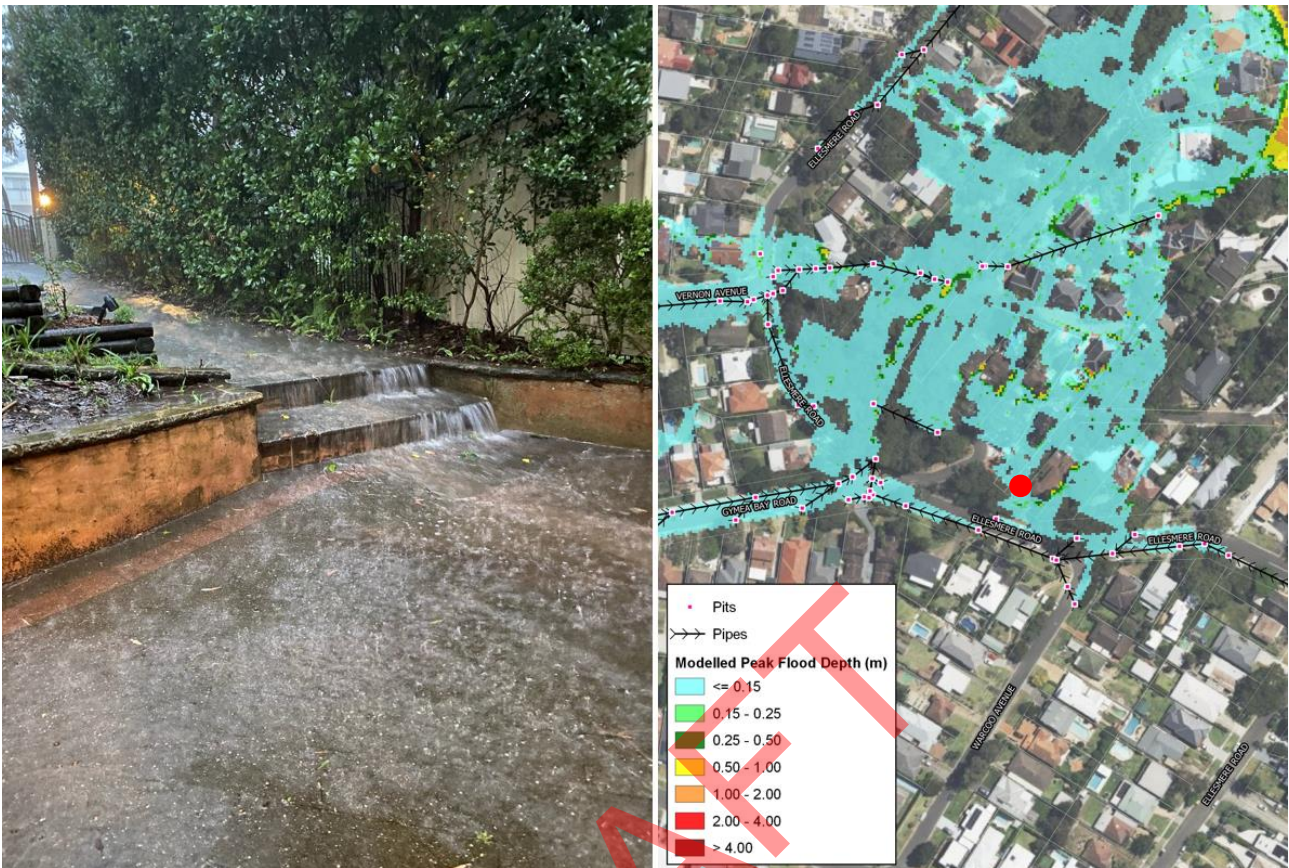
Figure 5.6 Photograph and Predicted Flood Depths for February 2020 Event – Ellesmere Road (GyMEA Bay)
