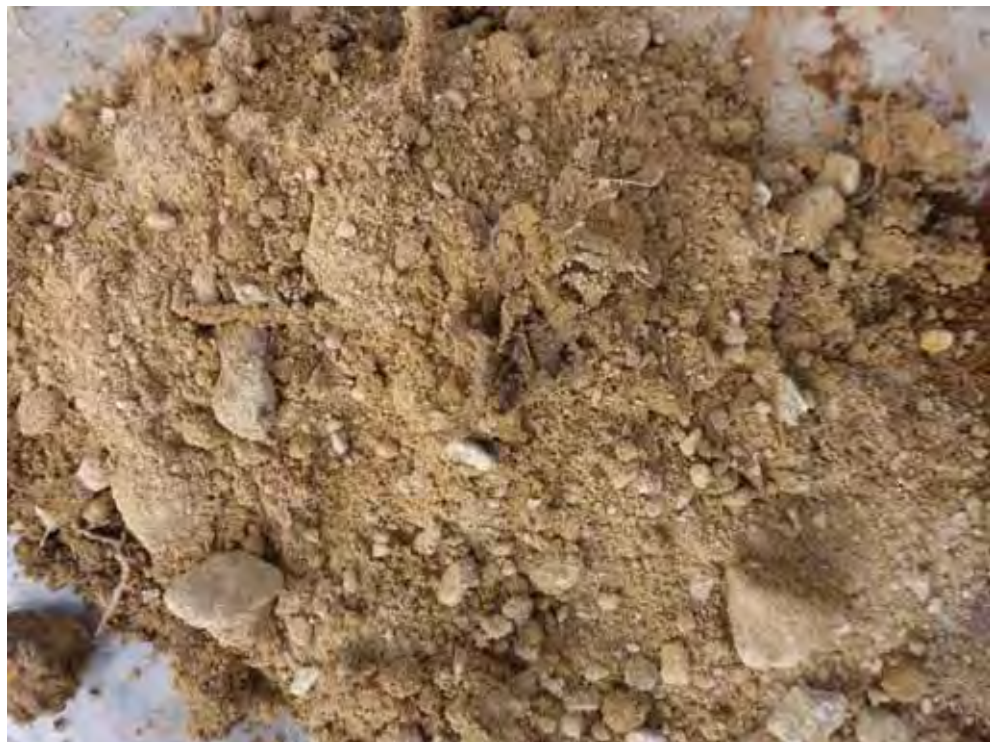
Photo 6 Gravelly sand fill material encountered at borehole BH32 between 0.22 m and 0.35 m (2/7/2019).
