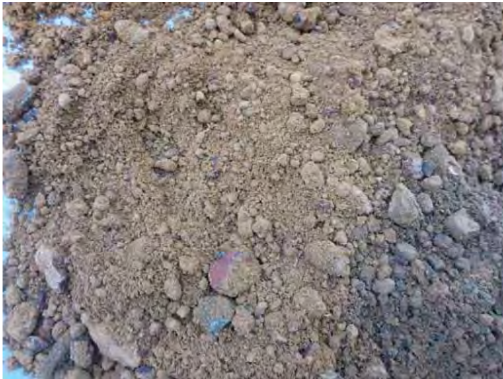
Photo 5 Silty gravel encountered at borehole BH26 between 0.20 m and 0.65 m (2/7/2019).
